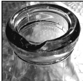
Figure 1 – Slot or notch in finish (Lillienthal 2003:2)
