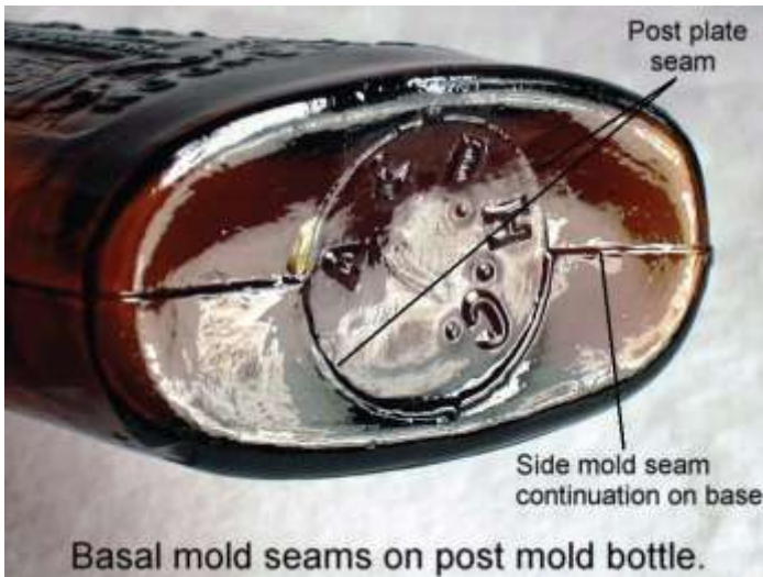
Figure 6b. Post-bottom mold produced bottle. The “post” seam is a result of a separate base mold section or plate. Bottle pictured is a Warner’s Safe Tonic (Rochester, NY), ca. 1879–1883 (Seeliger 1974). (Photo by Bill Lindsey, 2005.)
