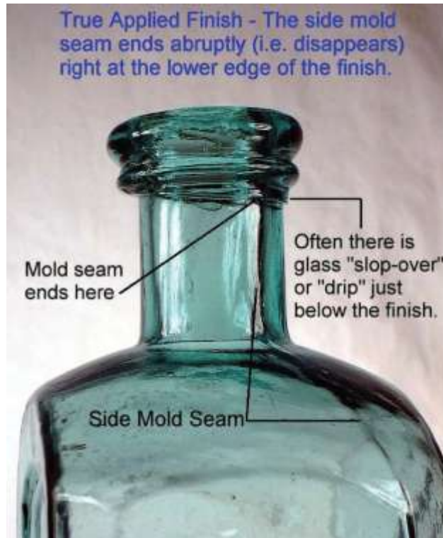
Figure 5. “True” applied finish (lip) with the side mold seam stopping abruptly at the base of the finish. Bottle is a Lindsey’s Blood Searcher (patent medicine from Hollidaysburg, PA), ca. 1855–1865. (Photo by Bill Lindsey, 2005.)
