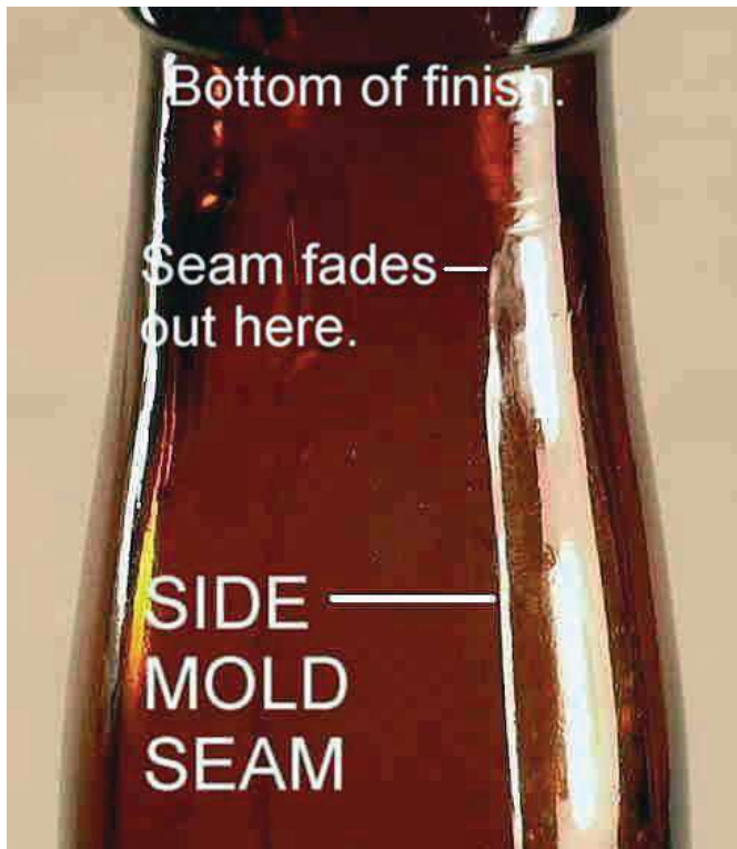
Figure 1. Vertical side mold seam on the neck of a beer bottle ending well below the tooled finish, indicating that it was at least partially handmade. This is a typical 11–12 oz. beer bottle, ca. 1905–1915. (Photo by Bill Lindsey, 2005.)
