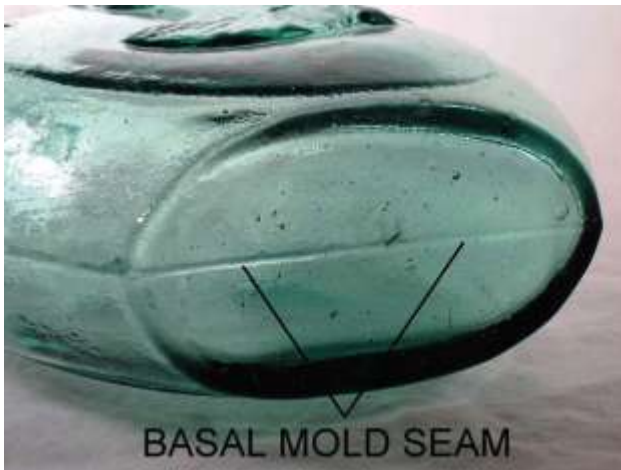
Figure 6a. Basal mold seam across the bottom of the bottle. Bottles produced in a simple two-piece mold with no separate base part have a mold seam that bisects the entire base. These are often referred to as hinge mold or snap-case bottles. This bottle is a Washington-Taylor figured flask (Philadelphia, PA), ca. 1860–1870. (Photo by Bill Lindsey, 2005.)
