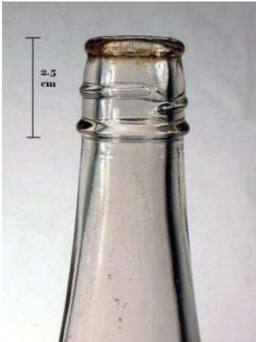
Figure 12. External (continuous) screw threads on a Heinz™ catsup bottle produced by the Illinois Pacific Glass Company (San Francisco, CA), ca. 1925–1930. (Photo by Bill Lindsey, 2005.)
