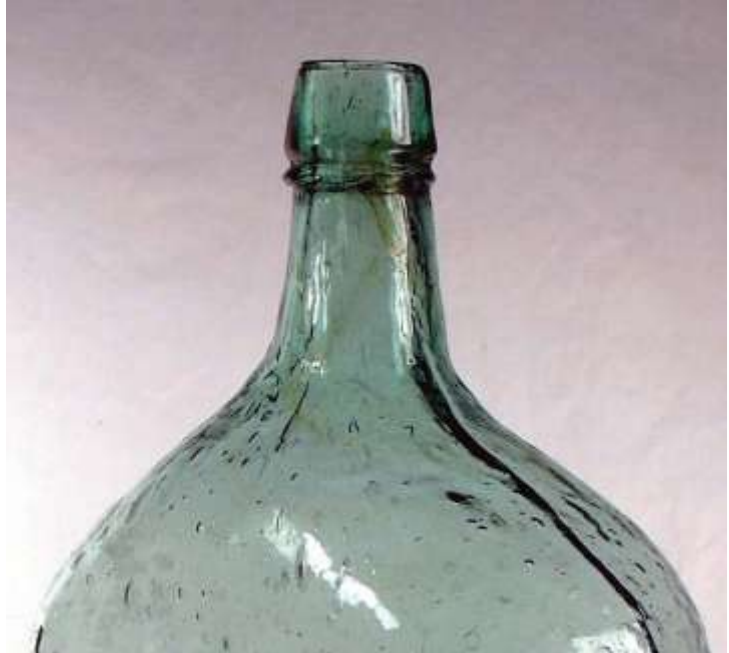
Figure 9. Bubbles in the shoulder glass of a bottle. This is an extreme example of the number of bubbles to be found in a bottle. (Photo by Bill Lindsey, 2005.)
