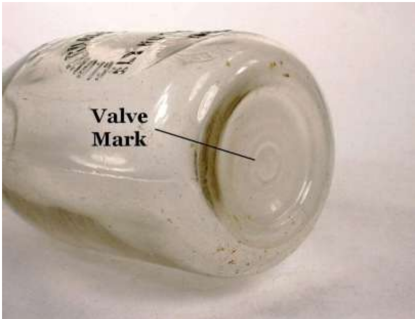
Figure 14. Valve mark on the bottom of a Cloverdale Dairy bottle, ca. 1925–1930. (Photo by Bill Lindsey, 2005.)
