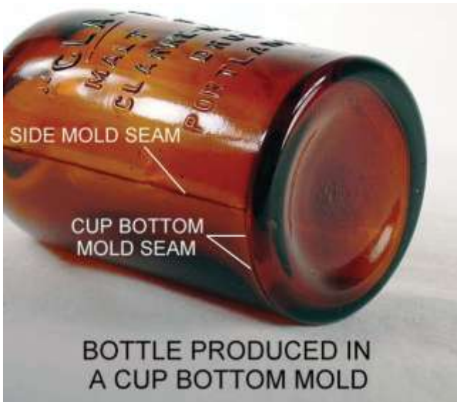
Figure 6c. Cup-bottom mold-produced bottle with no mold seams within the base. Bottle pictured is a Cla-Wood Malt Tonic from Portland, OR (White 1974), ca. 1906–1916. (Photo by Bill Lindsey, 2005.)
