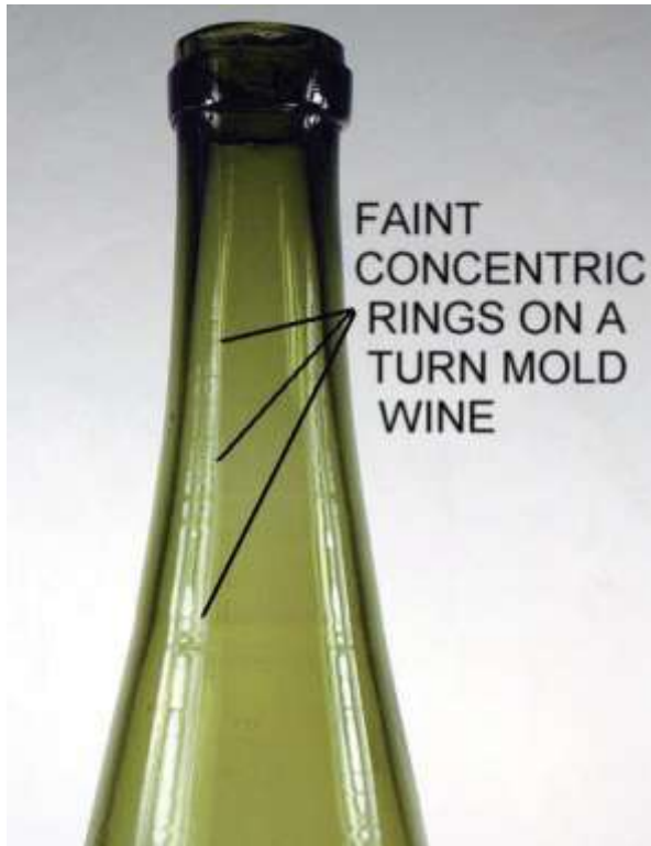
Figure 3. “Hock” wine bottle, ca. 1890–1915. The concentric rings are not always as obvious as the picture shows and sometimes not visible. Although if present this characteristic is a conclusive diagnostic feature. (Photo by Bill Lindsey, 2005.)
