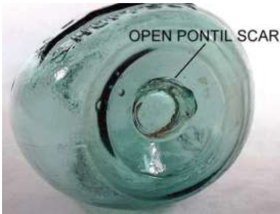
Figure 4. Examples of the three major pontil types: (a) glass-tipped or “open” pontil scar on a pictorial calabash flask from Isabella Glass Works, NJ, ca. 1850–1855; (b) iron or “improved” pontil scar; and (c) sand (disk) pontil scar on a “Rickett’s Patent” liquor bottle, 1822 (this bottle has a dated blob seal). (Photo by Bill Lindsey, 2005.)
