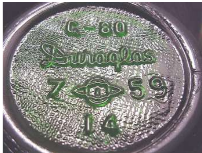
Figure 17. Stippled base on the bottom of a 1959 soda bottle. (Photo by Bill Lindsey, 2005.)
