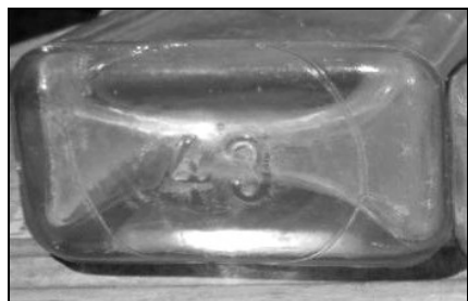
Figure 40 – Fletcher base with machine scar and "43" (eBay)
