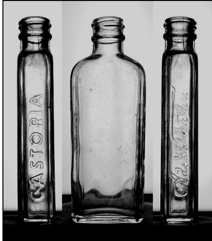
Figure 44 – Second bottle with continuous-thread finish
