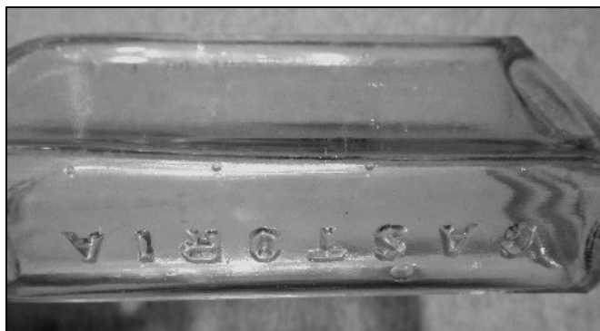
Figure 70 – Vent marks on a side panel of Dr. Pitcher’s bottle
