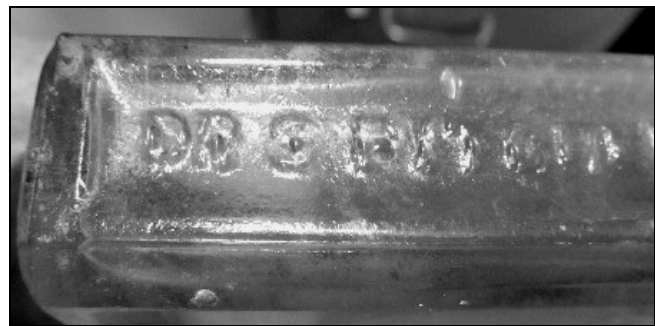
Figure 28 – Vent marks concealed in embossed letters
