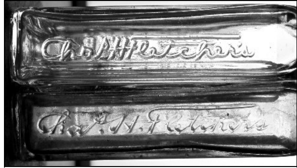
Figure 33 – Slight differences in font between mouth-blown and machine-made Fletcher bottles
