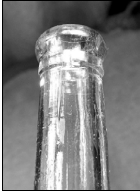
Figure 25 – Closeup of tooled finish on PITCHER’S bottle
