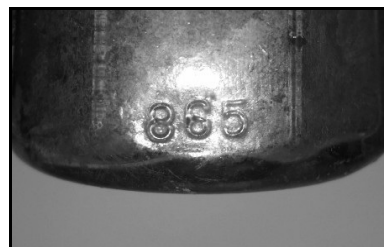
Figure 8 – mold number heelcode
