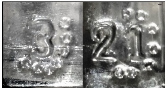
Figure 7 – heelcode – circle of dots around number
