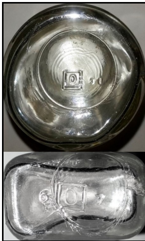
Figure 5 – Placement of plant and date codes
